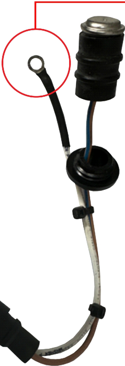
0585185 – Substitute Temp Switch (After Modification – Installed)
